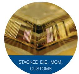
Ultra low loops (<1.5x dia); cantilevered die stacks
