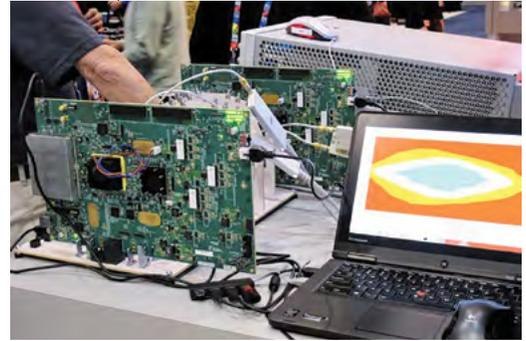
Teraspeed® Consulting demonstration of a 28 Gbps backplane system attaching two Xilinx VCU109 Evaluation Boards across Samtec's ExaMAX® backplane connectors. The demo leveraged advanced design optimization techniques that minimize insertion loss, return loss and crosstalk, while utilizing advanced PCB materials. Photo courtesy of Xilinx.
