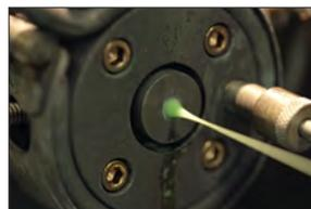
Precision extruded micro coax and twinax cables
